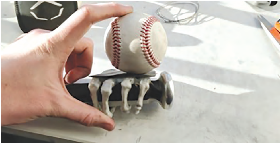
Undergraduate Nigel Archer builds a human hand model to test ball impacts.
